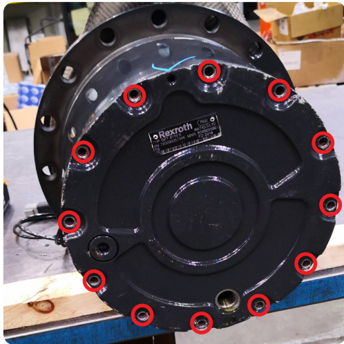
Unscrew the 12 screws that secure the cover.
